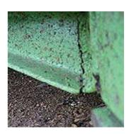
Under the cyclic loading conditions and typical stresses encountered by lifting equipment, this kind of starter crack can eventually propagate (a process called "fatigue crack growth") to the point where it will be detectable via nondestructive testing.
